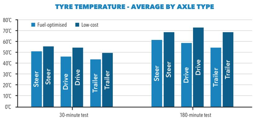
day; low-cost tyres the second. During these trials, an identical control truck fitted with a single set of tyres shadowed the trial rig. To cancel out differing track conditions - and the wind picked up on the second day - results were modified ('normalised') by factoring in fuel performance variations between the runs of the control truck.
